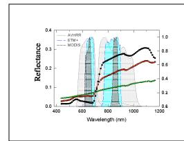
Figure 1. MODIS, Landsat ETM+, and NOAA-AVHRR normalized bandpass filters superimposed onto three hyperspectral reflectance signatures (Miura et al., 2002).
