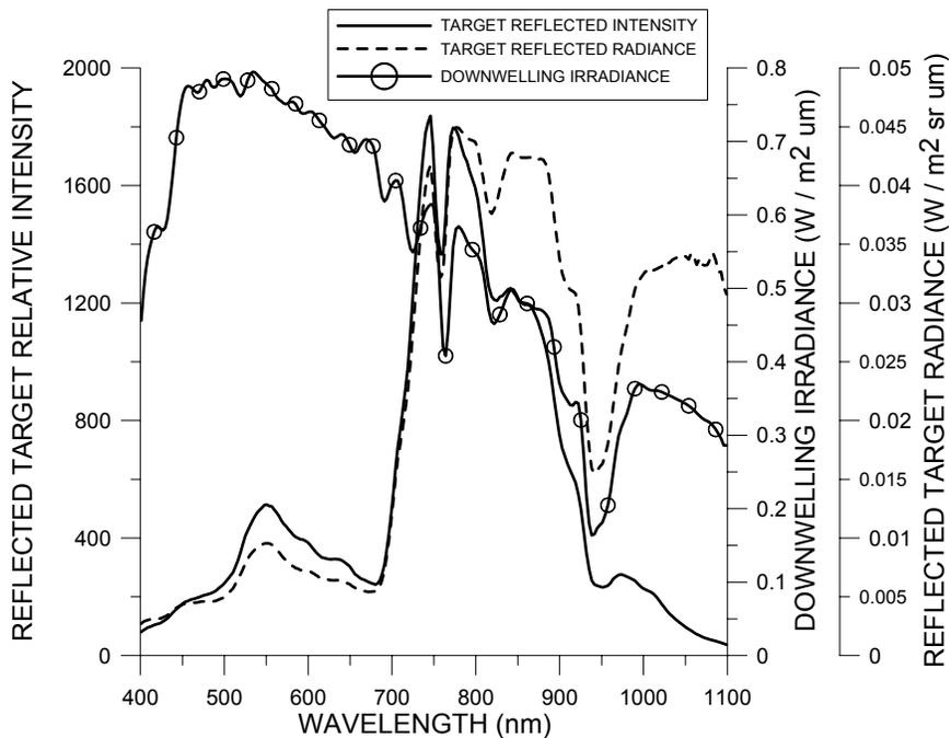
**Figure 3. Measured downwelling irradiance at the time of the Hyperion image data collection. Measured upwelling intensity before and after calibration to radiance. Absorption features associated with water (about 930 nm to 960 nm) and oxygen (around 690 nm and 760 m) are shown in the recorded spectra.**
