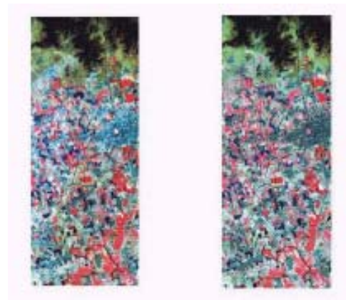
Figure 3. False-color composite imagery near Beijing City, China, before (left) and after atmospheric correction.
