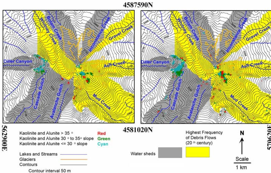
Figure 3. AVIRIS (left) and Hyperion identification of steep altered bedrock areas.
