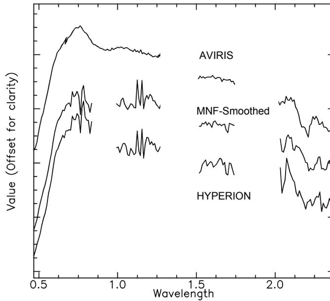
Figure 2. Image spectra from the same ground location.
