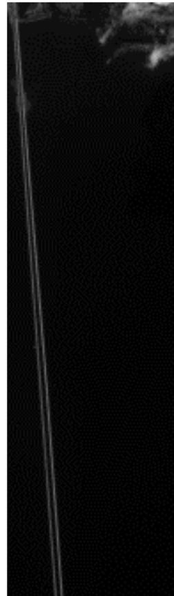
**Figure 2. Lake Pontchartrain Causeway was used to analyze the ALI 10-meter panchromatic band in the cross-track direction. These results were compared to the spatial response of ETM+.**
