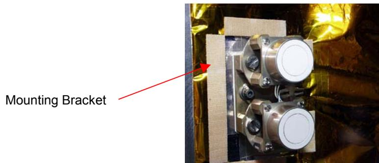
**Figure 1. Flight Calorimeters**
