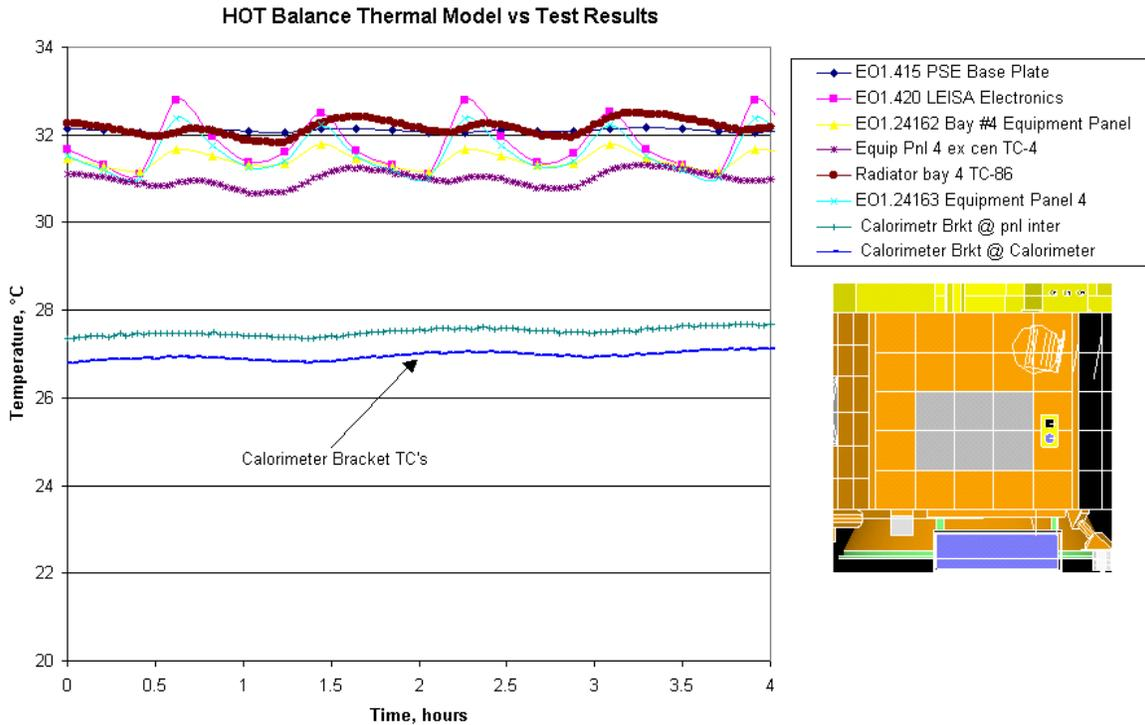
**Figure 3. Thermal Model Ground Test Correlation**
