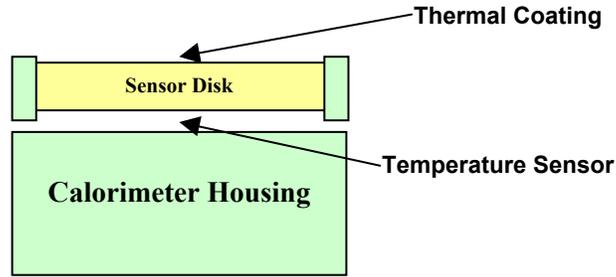
**Figure 2. Relationship Between the Calorimeter Sensor Disk and Housing**
