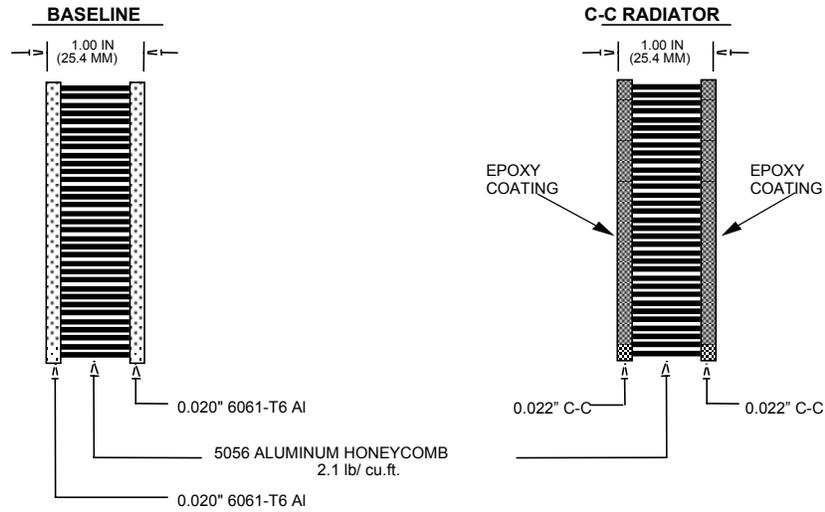
**Figure 3. Carbon-Carbon and Baseline Cross-Sections**
