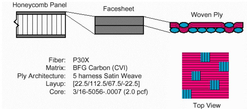
**Figure 4. Carbon-Carbon Radiator Facesheet Construction**
