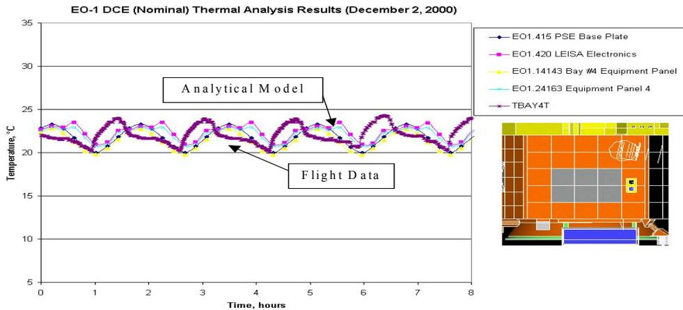
**Figure 7. Comparison of Flight Data with Analytical Model Data**
