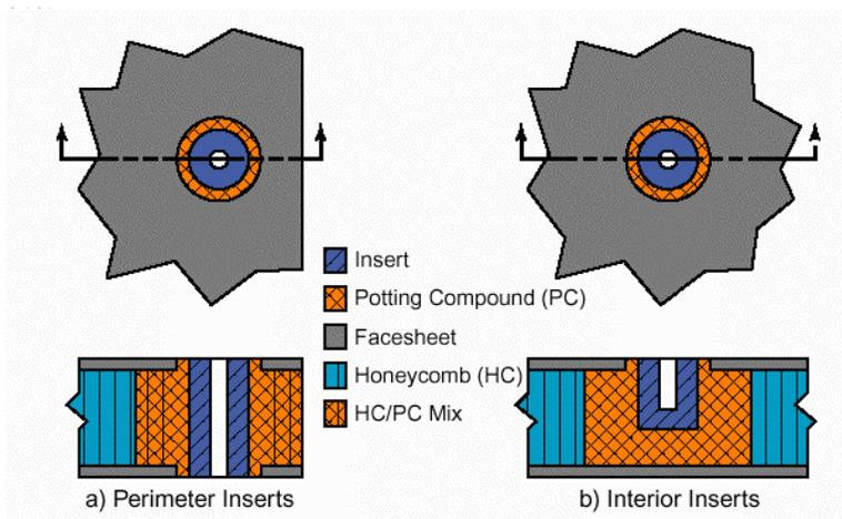
**Figure 5. Carbon-Carbon Radiator Panel Insert Design**
