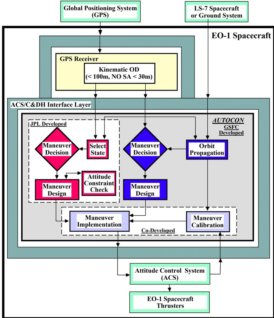
**Figure 1. EO-1 EFF Flight Software Architecture (JPL Approach)**
