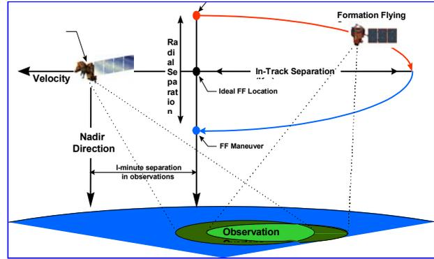
**Figure 2. EO-1 and Landsat 7 Formation Geometry**
