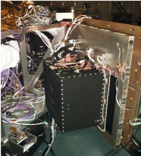
**Figure 1. WARP Mounted in Bay 1 of EO-1 Spacecraft**
