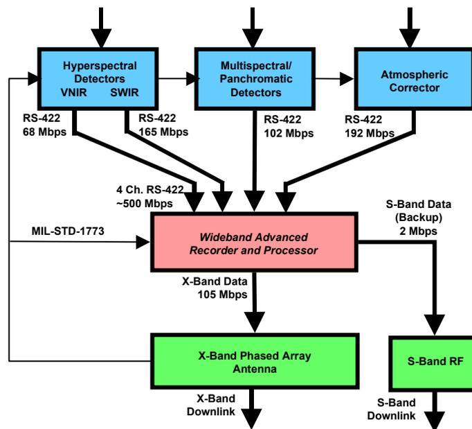
**Figure 3. EO-1 Flight Data System Architecture**
