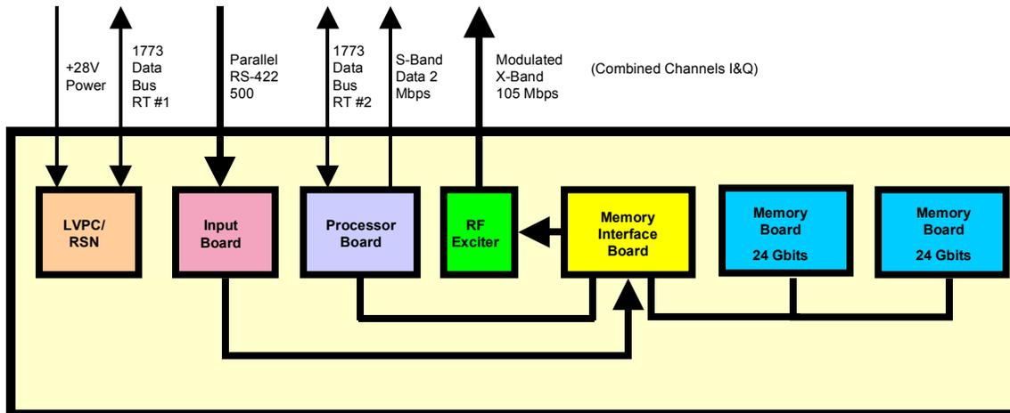
**Figure 4. WARP Hardware Architecture**
