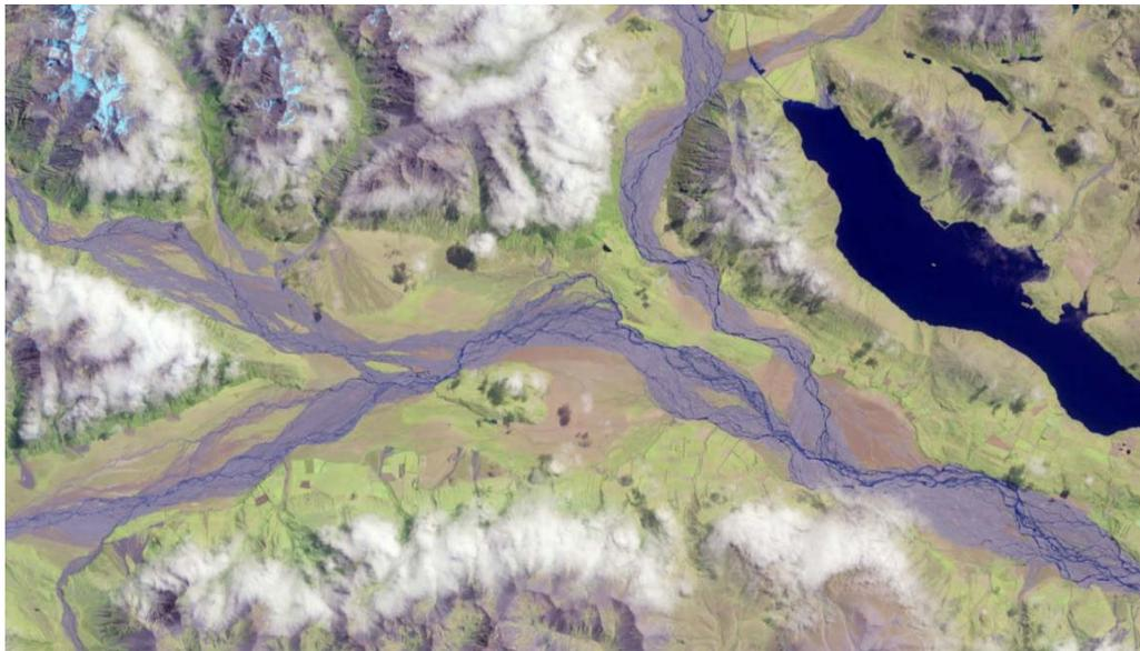
**Figure 3. False-color multispectral image of part of the South Island of New Zealand. Seen here are parts of the Rolleston Range, Lake Coleridge, and the Rakaia River. The red, green, and blue components represent Bands 7, 4, and 2, respectively. In this presentation, snow on the mountain peaks appears light blue, while clouds near the peaks are white.**
