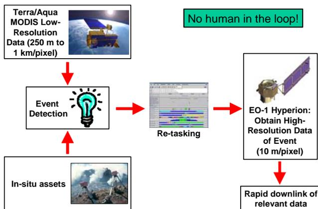
Figure 1. Sensorweb Detection and Response Architecture
