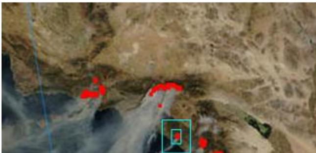
**Figure 5:** Active fire alerts for the recent October 2003 Southern California Fires. Red indicates active fires. The light blue box illustrates the background region used in the relative threshold detection.
