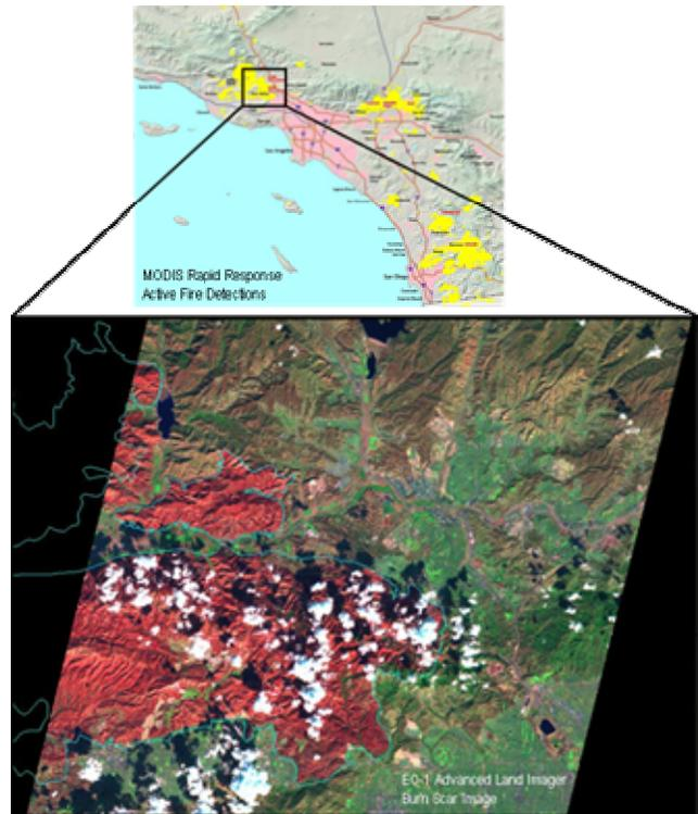
**Figure 6:** Sensorweb trigger images for October 2003 Southern California Fires. Above is the MODIS Active Fire Map display. Below is the EO-1 Hyperion image acquired via sensorweb trigger of the Simi/Val Verde fire area used in Burned Area Emergency Reclamation (BAER).
