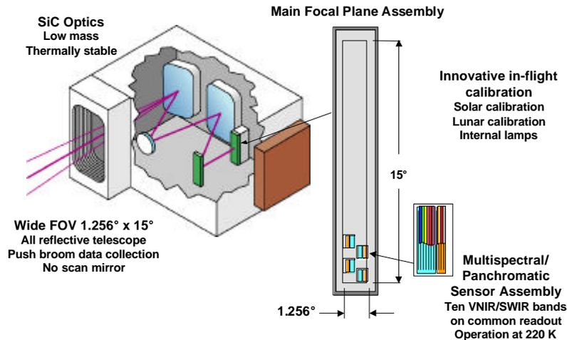
Figure 2. A conceptual sketch of the ALI telescope and Focal Plane Assembly.
