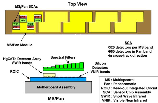
Figure 4. Focal Plane Assembly.
