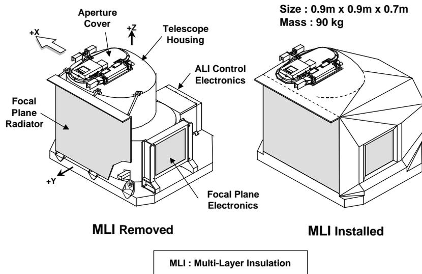
Figure 1. ALI instrument configuration showing the main thermal, mechanical, and electronic components.
