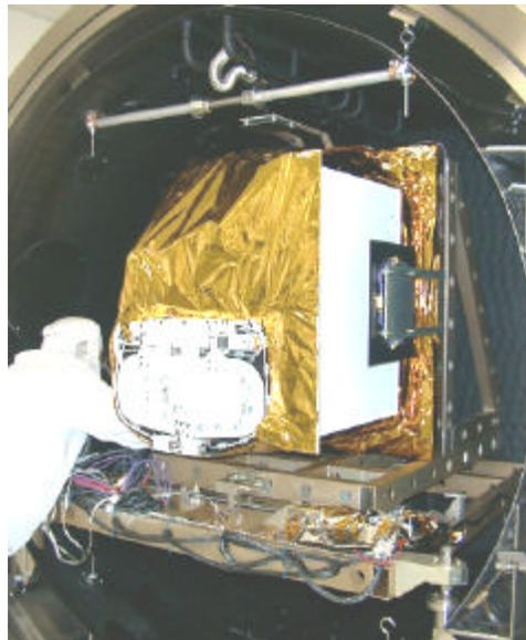
Figure 6. ALI being placed into thermal-vacuum test chamber.
